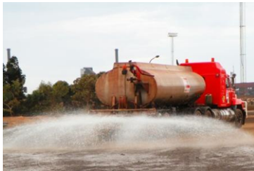
Water tankers are used to apply water/chemical dust suppressants to sites within an area of operations that has the potential to generate dust including unsealed roads, haul roads and dump areas.
