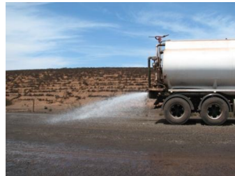
Water tankers are used to apply water/chemical dust suppressants to sites within an area of operations that has the potential to generate dust including unsealed roads, haul roads and dump areas.
